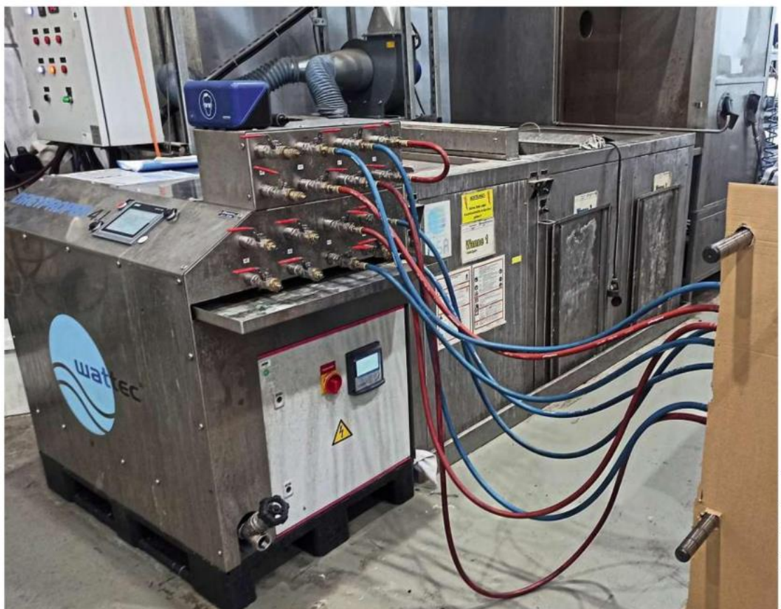
The Dreyproper injects air bubbles into the volume flow of the cleaning agent so that even stubborn limescale and sludge deposits can be removed.
